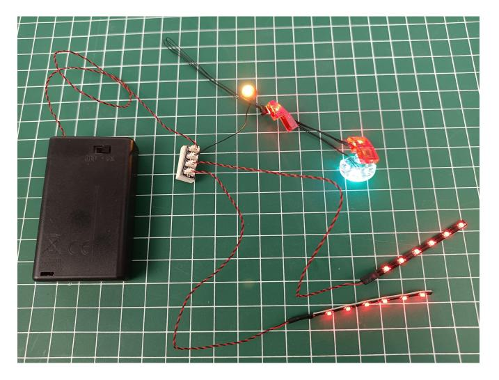
Turn off the power switch and separate the AAA Battery Pack from the 4-Port Expansion Boards.
